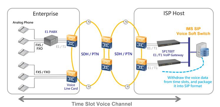
To adapt to the trends of networking and IP-based communication, TAINET has developed an E1/ T1 ISDN Trunking Gateway that can operate in SDH/ PTN bearer network environments. This gateway extracts voice streams, encapsulates them in SIP format, and registers the voice data with IMS (IP Multimedia Subsystem) voice softswitch systems or enterprise IPPBX voice softswitch systems.
